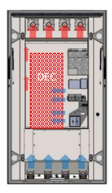
Fan Group 2 [Optional – Secondary] Low pressure / capacity exhaust fans run at a speed calculated to match the volume intake of feeder fans, and balance airflow through the
